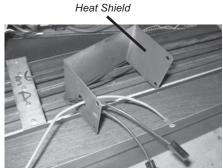
Plug the DC spark generator wires to the DC Sparker.
